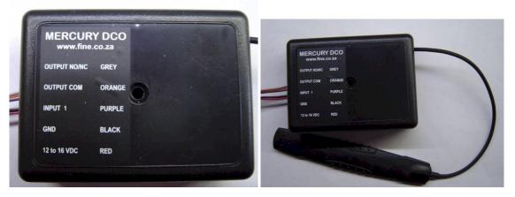
The Mercury can operate on Pre Paid or Contract SIM cards and when used on Pre Paid will SMS balance daily or can be set to SMS balances every from 1 to 30 days.
