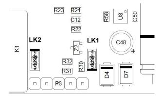
LK2 is used to change the relay from Normally Open to Normally Closed.
