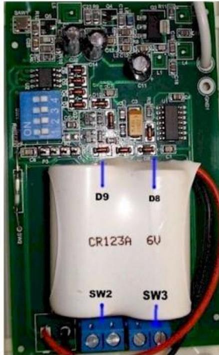
**SW2 is the normally Closed input for a magnetic Switch.
